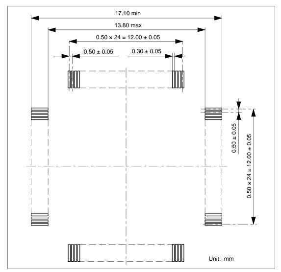
Figure 4 Recommended Dimensions for Mount Pad
